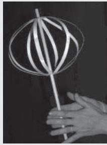
Fig. 11: Model to simulate flattening due to rotation.
